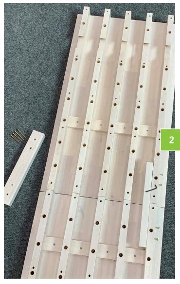
Lay myWall panels face down on a clean floor. Place both top and bottom sections next to each other. Top section has the cut-outs for the french cleat mounting at the top. The bottom panel has a lower open section at the bottom.
