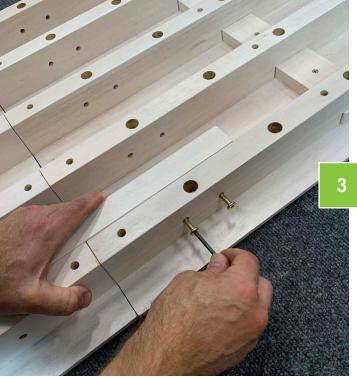
Attach connector blocks to fasten top and bottom of your myWall panel together.
